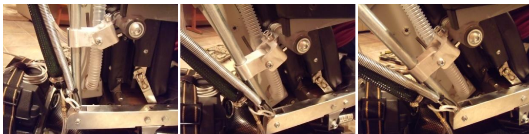
Figure 48. Incremental images of angle change during wheelchair recline.
