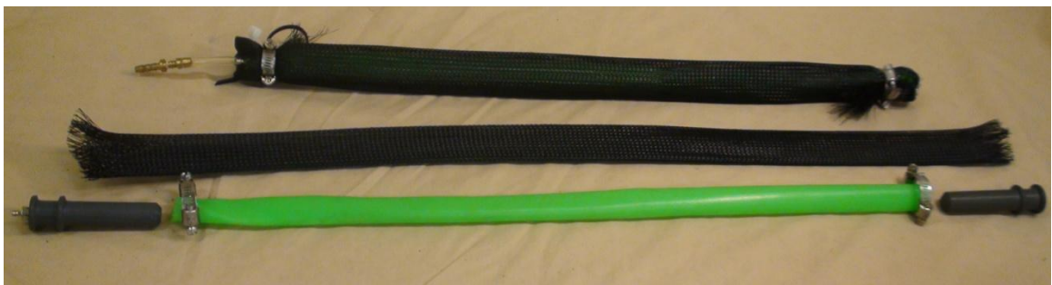
Figure 28. Complete air muscle (top), air muscle components (bottom).
