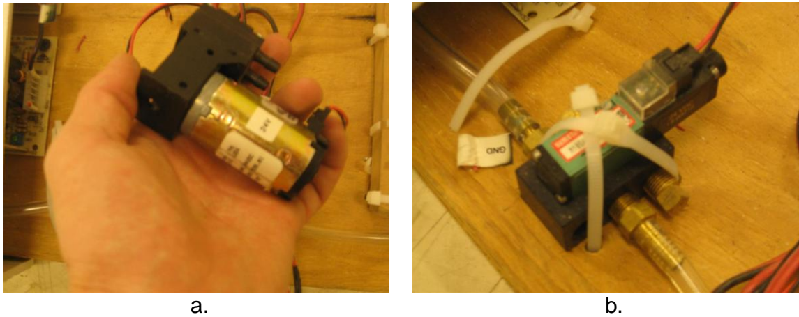
Figure 29. 24V air pump and electronic air release valve.
