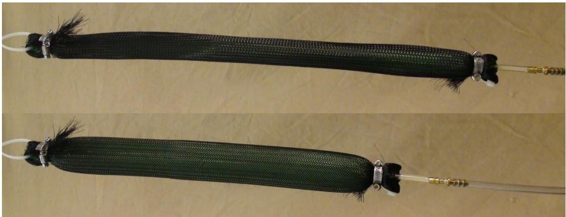
Figure 30. Air muscle deflated (top); air muscle inflated (bottom).
