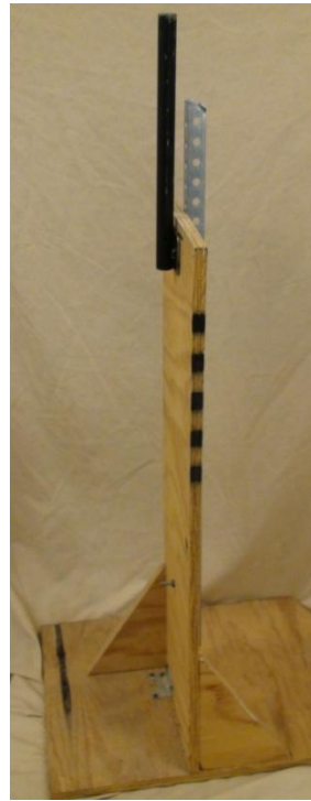
Figure 31. Testing rig with female mounting bracket attached.
