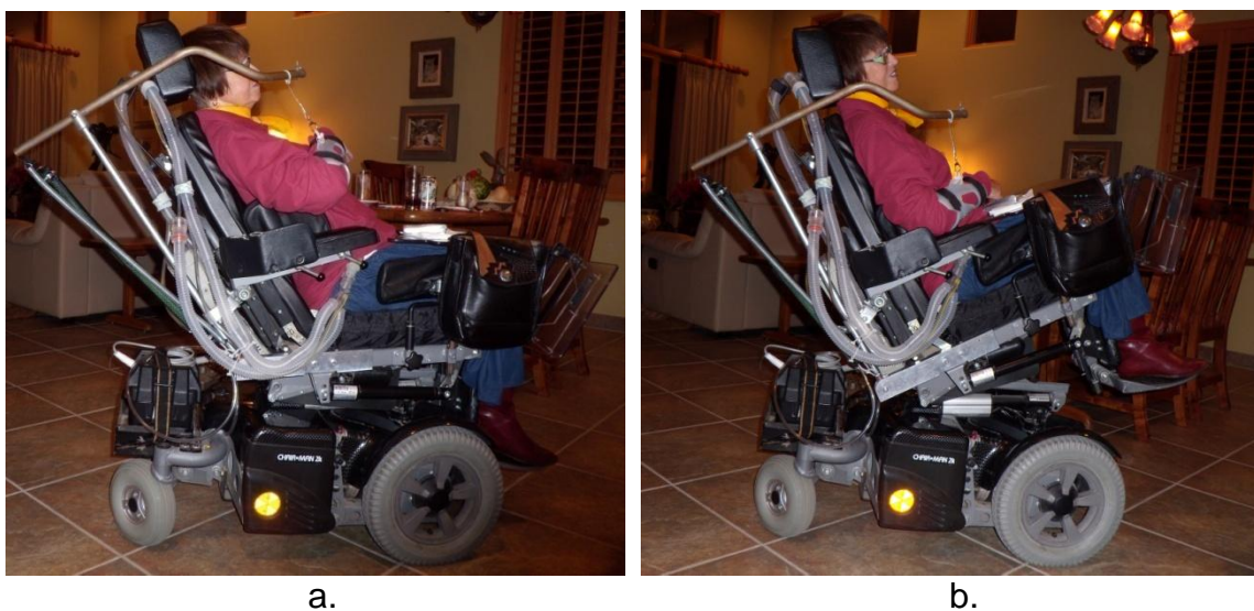
Figure 49. With PAL attached, wheelchair can still recline and tilt back.
